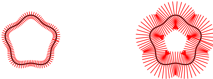
Figure 1: The condition number \Delta(M) of a manifold is the largest number \kappa such that the normals to the manifold do not cross as long as they are not extended beyond \kappa . The plot on the left shows a one-dimensional manifold (a curve) and some normals of length r < \kappa . The plot on the right shows the same manifold and some normals of length r > \kappa .
